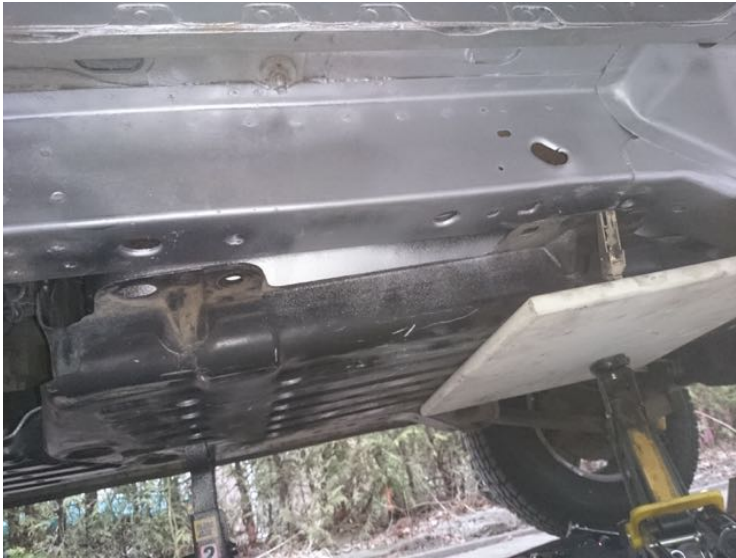
Support armour and tank with jack stands, jack etc before releasing bolts
