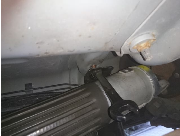
Difficult to reach front 18 mm passenger side bolt does not require removing drive shaft if you have right wrench
