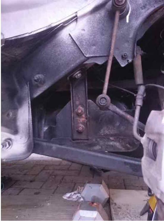
Driver's side rear wheel bracket. This is the rusted corner.
