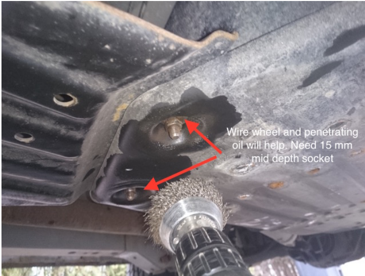
Penetrating oil and a wire wheel will make these 15 mm nuts easier to take off with a deeper than normal socket
